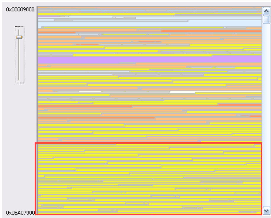
Figure 4: Yellow blocks are my chunks of data sprayed with JS. The other segments are other informations stored by the browser
